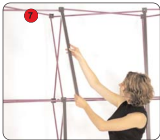
7. Place the channel bars onto the frame.
